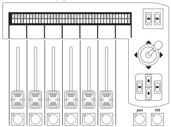
Above each fader, the display indicates the effect it's controlling and the value set. Pressing one of the buttons, control is assigned to the four cursor arrows. When Pan and Tilt are lit, the cursor controls the positioning of the effects fixtures' mirrors and heads.
