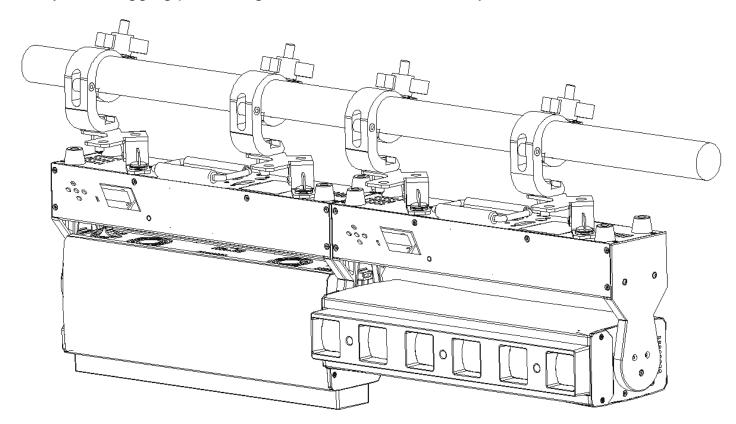
Regardless of the rigging option you choose for your LED pixel Zoom bar 240, always be sure to secure your fixture with a safety cable. The fixture provides a built-in rigging point for a safety cable on the hanging bracket as illustrated above. Be sure to only use the designated rigging point for the safety cable and never secure a safety cable to a carrying handle.
